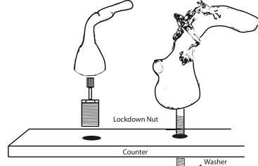
If applicable, turn off the water supplies and remove the old faucet and drain. Drill 3 holes, each 1 1/4" in diameter, for the spout and valves.
