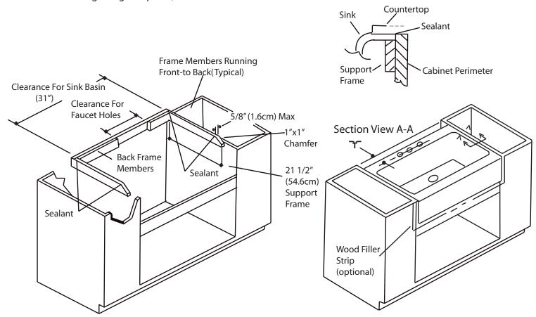
There should be a hole cut in the front of the cabinet face to accommodate the apron front as well. Measure sink apron and cabinet opening to make sure apron will fit into cabinet opening. If necessary, sand opening or add wood filler strips. Apron should rest against the cabinet face. This sinks apron can protrude 2 - 2 1/4" away from the cabinet wall, **NOTE you MUST measure to accommodate this variance to determine actual hole depth for sink as well.**
