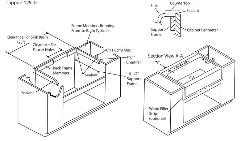
There should be a hole cut in the front of the cabinet face to accommodate the apron front as well. Measure sink apron and cabinet opening to make sure apron will fit into cabinet opening. If necessary, sand opening or add wood filler strips. Apron should rest against the cabinet face. This sinks apron can protrude 2 - 2 1/4" away from the cabinet wall, **NOTE you MUST measure to accommodate this variance to determine actual hole depth for sink as well.**
